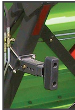
Rubber bumpers for dumping into trucks.
