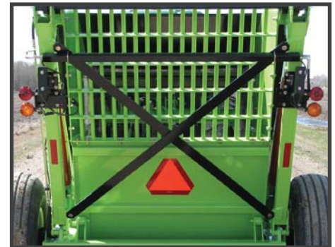
Round bar grated back bucket. High Rise 8000 only
