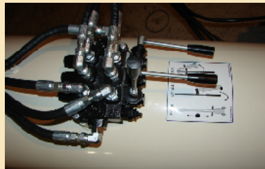
3-Way Control at the hopper
