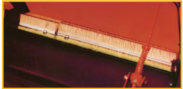
Brush Agitators - keep the seed flowing at a positive, accurate rate and provide instant shut-off the moment the seeder is stopped; prevents seeding "skips" and bunching of seeds.
