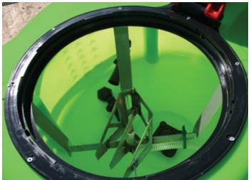
**Mixing:** two agitator jets stir the fluid while the four vertical ribs disrupt the flow increasing the rate of mixing and virtually eliminating the chances of undissolved particles.
