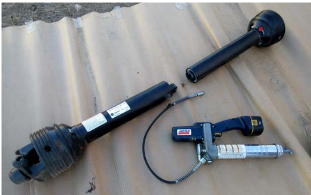
FIG. 80 TELESCOPING SECTION (TYPICAL)
