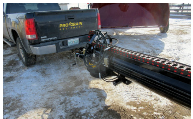
FIG. 20 TRUCK TRANSPORTING (TYPICAL)
